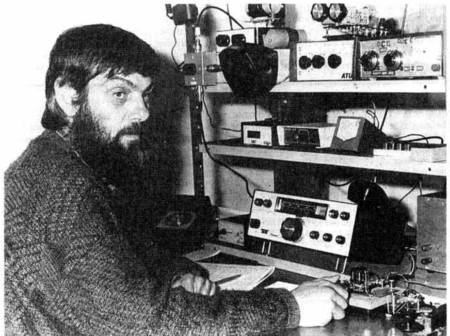
G3RJV ON QRP DAY FROM ST. AIDAN'S CHURCH, ROCHDALE. TRANSCIVER WAS AN ARGONAUT 509 (2 WATTS) WITH AN ERA BP34 CW FILTER, PLUS HOME-BUILT KEYS AND ATU S. (PHOTO ROCHDALE OBSERVER).
